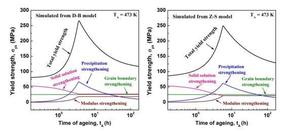
Contribution of various strengthening mechanisms to total yield strength of AA 6063 alloy aged at 473K simulated from both D-B and Z-S model.
