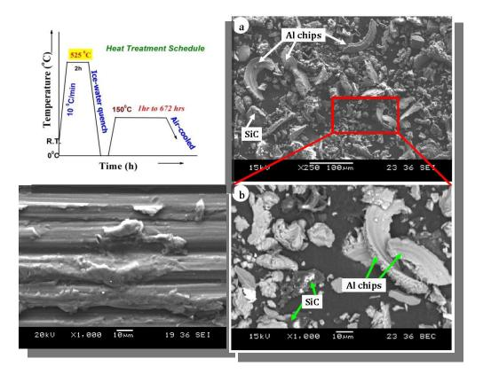
Illustration of Heat treatment Schedule and Images of worn pin surface and wear debris at ageing temperature of 150°C for 8h
